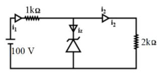
For zener breakdown, potential difference across  $2k\Omega$  resistor will be 5.0 V
